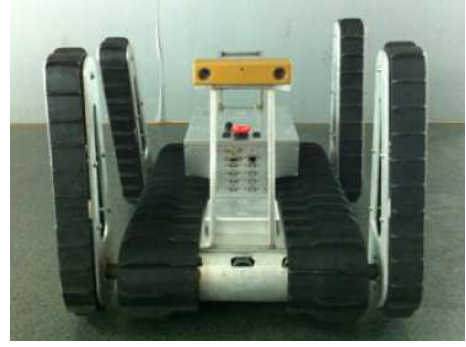
Fig. 5. The NuBot rescue robot equipped with a Bumblebee2 stereo vision system.
