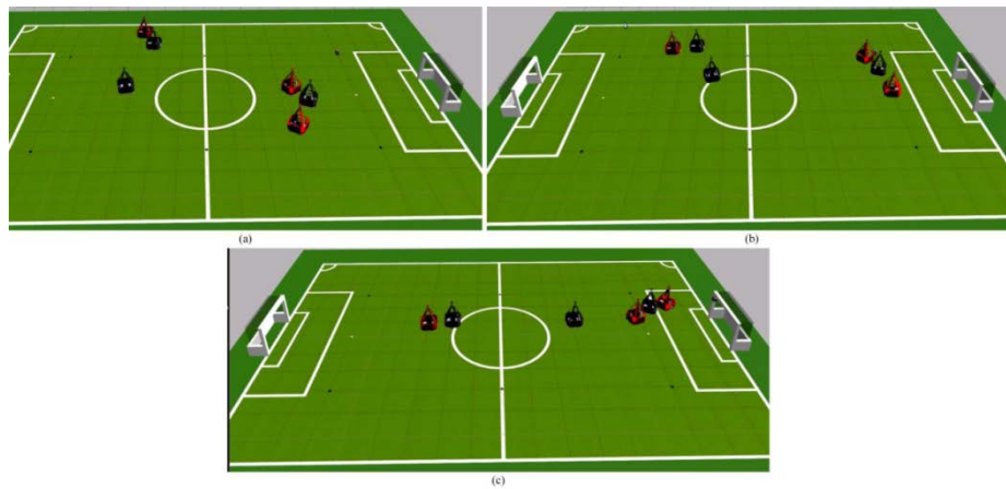
Fig. 8. Two sides of robot models compete in a soccer game. (a) The initial state of the robot models (black) and the rival robot models (red); (b) three robots on the right side of the soccer field are chasing the soccer ball; (c) Black robots shoot the goal.
