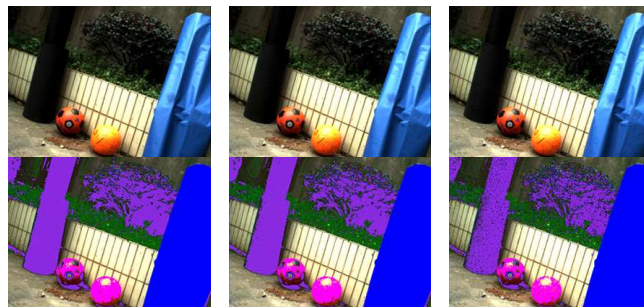
Fig. 4: The typical images along the ridge curve and the processing results in outdoor experiment. (top) are the typical images. (bottom) are the processing results. The camera parameters are as follows: (left) exposure time: 22ms, gain: 9. (middle) exposure time: 14ms, gain: 14. (right) exposure time: 7ms, gain: 22.
